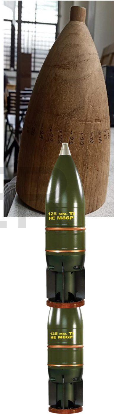
Figure 4: Dummy wooden model and the original 125 mm HE projectile
